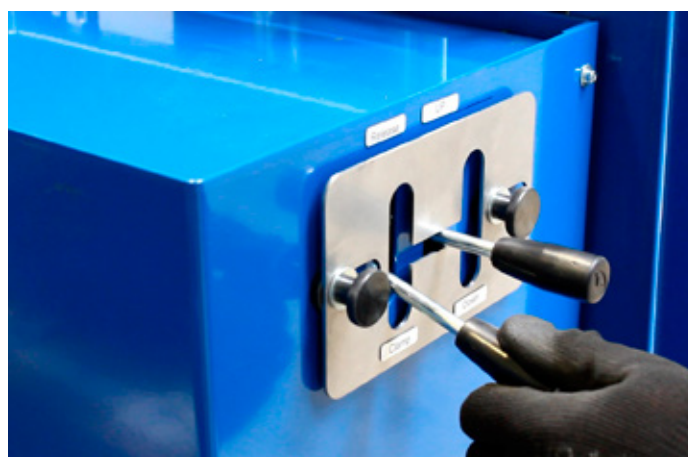
Levers for wheel clamping and lifting/lowering
