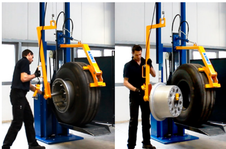
C-Hook for easy removing of heavy rim parts
